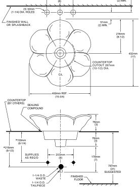
NOTES: \*DIMENSIONS SHOWN FOR LOCATION OF SUPPLIES AND "P" TRAP ARE SUGGESTED. FITTINGS NOT INCLUDED WITH FIXTURE AND MUST BE ORDERED SEPARATELY. FOR COUNTERTOP CUTOUT AND INSTALLATION INSTRUCTIONS USE TEMPLATE SUPPLIED WITH LAVATORY.
